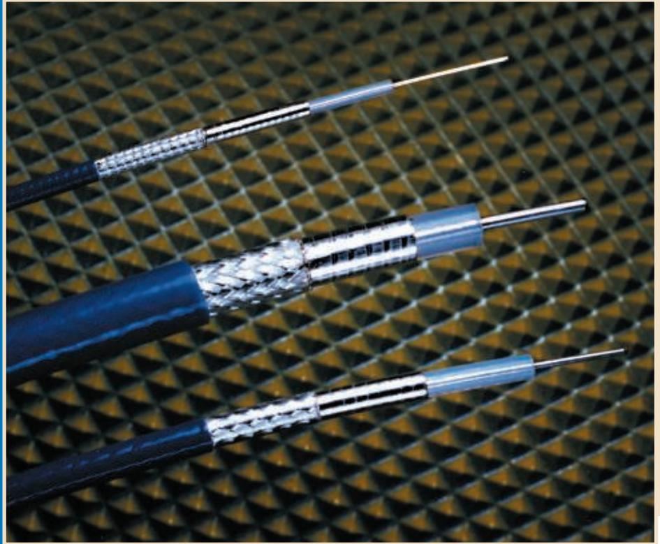
Developed over ten years ago as a lighter weight, flexible alternative to semirigid coax, TFlex<sup>®</sup> has been widely adopted for both military and commercial communication systems. Its Teflon FEP jacket provides excellent protection in corrosive environments and its flexible nature eliminates the need for hand or precision machine bending. Following the most convenient routing, TFlex<sup>®</sup> can be preterminated to its desired length and can then be just “plugged in”.
